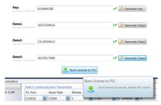
Once the licence has been successfully burned onto the PLC this dialogue box will appear showing that the Licence has been successfully sent to the PLC and it is now licensed. No further action is required.
