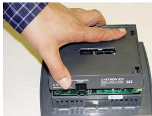
**Re-installing a Snap-in I/O Module**
