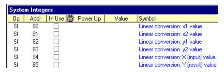
The linearization values created here can be displayed by linking SI 85 to a Display; the value **can** be used elsewhere within the project for further calculations or operations.
