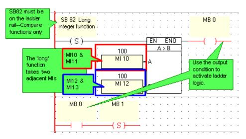
You can use the Store function in two ways; these can enable you to display long values on the LCD. Note that in order to display long values, the variable used to represent the 'low' byte should be configured to show leading zeros. Display is restricted to positive values within the range of 0-99,999,999.
