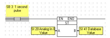
In the next net, the value in SI 40 is incremented by 1 every second, changing the current database integer. This means that the first analog value will be stored in integer 0, the second analog value in integer 1, and so on.
