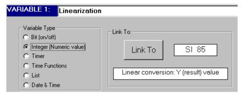
Example: write the variable ranges into SI 80 - 83, then writing an analog input into SI 84:
