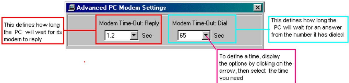
**Figure 5. Adjusting Time-out Settings**
