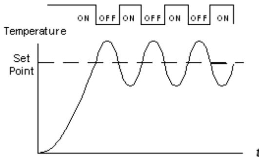
PID control enables you to minimize overshoot and damp the resulting
