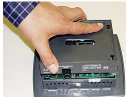
**Re-installing a Snap-in I/O Module**
