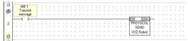
The PLC then monitors the COM port for a reply from the XYX robot and disassembles the message to place only the required data where you want it.
