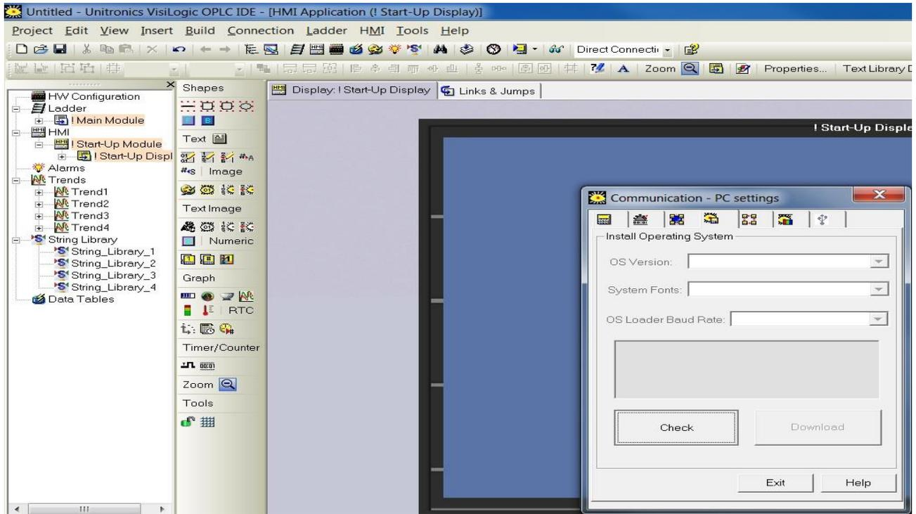
1. To install the new OS into the PLC, press Ctrl+F9 to open the 'Communication' window
