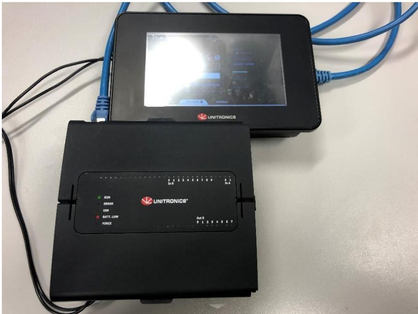
6) **Configure HMI panel IP Address** – Please note that both the HMI has a **Panel IP** address and the PLC has a different **Panel IP** address. The HMI subnet must match the subnet of the PLC in Network (i.e. If PLC panel IP = 192.168.1.XXX then HMI panel IP must = 192.168.1.XXX but not be identical to any other IP on the same network) With a subnet mask of 255.255.255.0 the first 3 digits of your PLC panel and HMI IP addresses must match. So, in our example –
